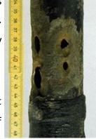
corrosion. In fact, at the point of entry, stray current provides certain degrees of cathodic protection to the metallic structure.
