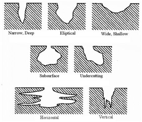
ASTM-G46 has a standard visual chart for rating of pitting corrosion.
