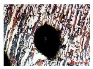
Pitting corrosion is usually found on passive metals and alloys such aluminium alloys, stainless steels and stainless alloys when the ultra-thin passive film (oxide film) is chemically or mechanically damaged and does not immediately re-passivate. The resulting pits can become wide and shallow or narrow and deep which can rapidly perforate the wall thickness of a metal.
