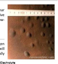
When hydrogen atoms meet in a trap and combine, they form hydrogen gas (H<sub>2</sub>) molecules in the trap. The accumulation hydrogen gas inside the extremely small cavity will lead to the buildup of excessive internal hydrogen pressure. At certain times, this internal hydrogen pressure will become sufficient to cause the steel to blister.
