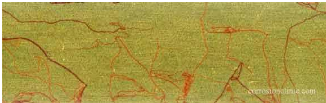
Filiform corrosion of a tin-coated steel
