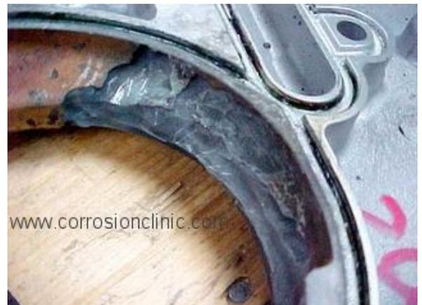
Erosion-corrosion is usually found at high flow rates around tube blockages, tube inlet ends, or in pump impellers. The photo shows erosion corrosion of a cast aluminum pump casing due to excessively high flow rate of the coolant.
