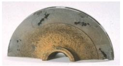
What is Cavitation Damage? Cavitation Damage refers to the degradation of a solid body resulting from its exposure to cavitation (This may include loss of material, surface deformation, or changes in properties or appearance).
