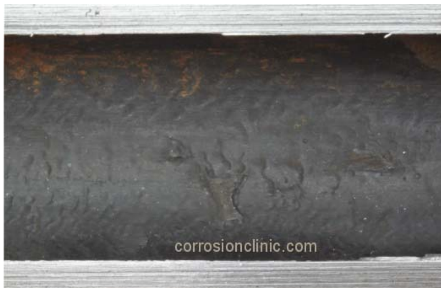
Figure 2b Erosion Corrosion showing classic pattern of erosion corrosion on the magnetite-covered tube ID surface
