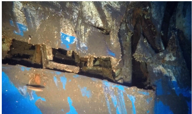
Figure 6. Horizontal/longitudinal crack/rift of Deck #3 located in between structural transversal frame #114 and #137.
