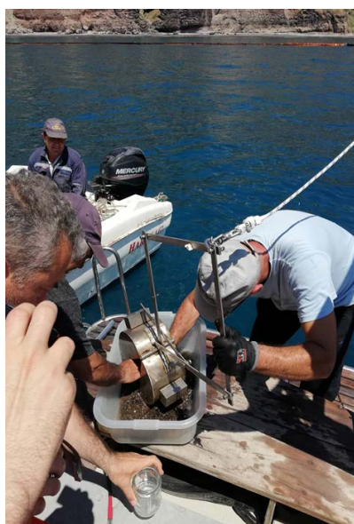
Figure 8. Grab sampler in action collecting seabed sediment (Thira island).
