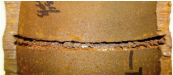
Figure 1 PWC-Compass Models and Predicts the Risk of Preferential Weld Corrosion.
