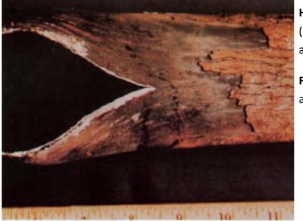
**CSR-Compass:** Modeling and Remaining Life Prediction of Creep and Stress High Temperature Creep and Stress Rupture Rupture of Boiler and Heater Tubes
