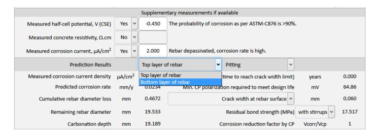
Figure 7 Concrete-Compass predicts corrosion of top layer and bottom layer of steel reinforcement in RC structures.
