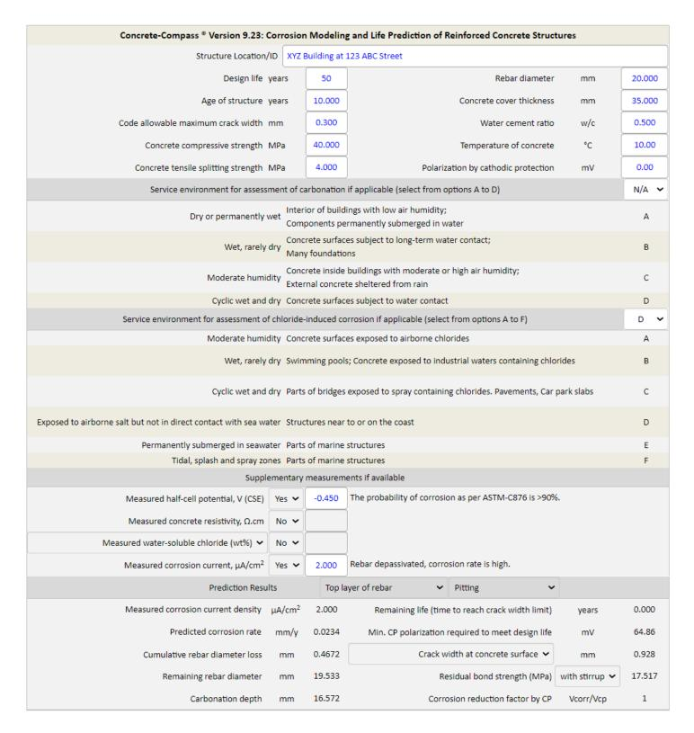
Figure 1 Concrete-Compass Predicts the rate of Concrete corrosion and the remaining life of RC structures.
