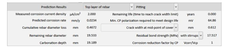
Figure 11 Concrete-Compass predicts the crack width at different depth of concrete cover, crack width at mid-point of cover.
