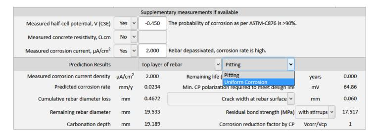
Figure 8 Concrete-Compass predicts the effect of corrosion types on the crack width and remaining life of RC structures.
