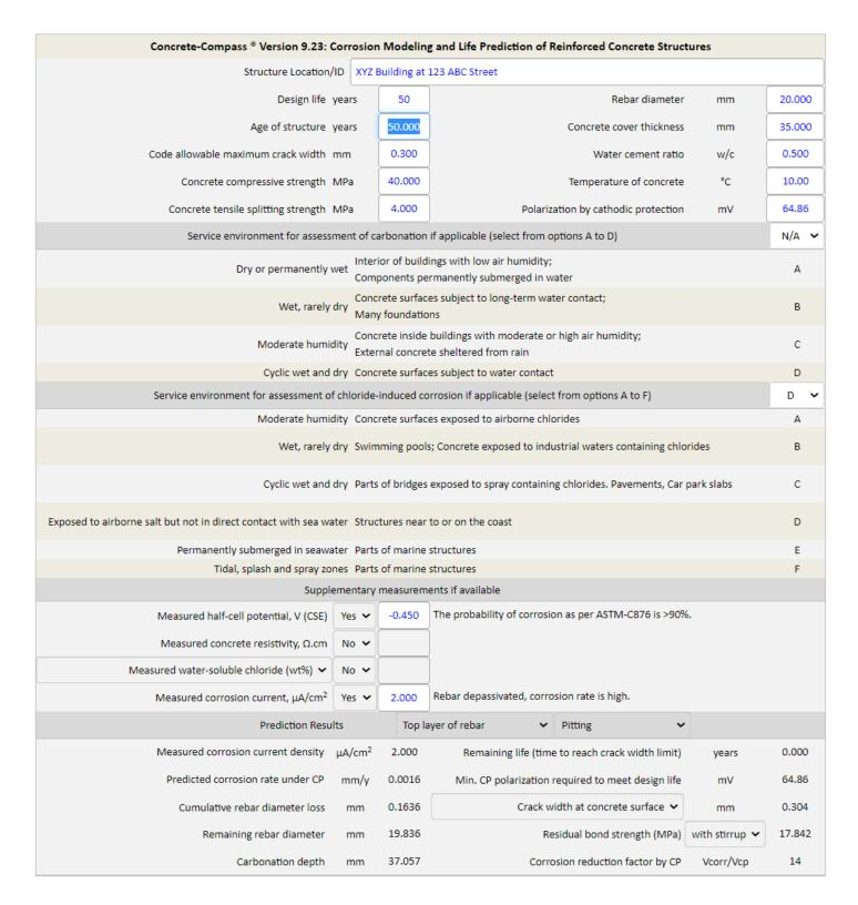
Figure 3 Concrete-Compass predicts concrete corrosion and effectiveness of cathodic protection.
