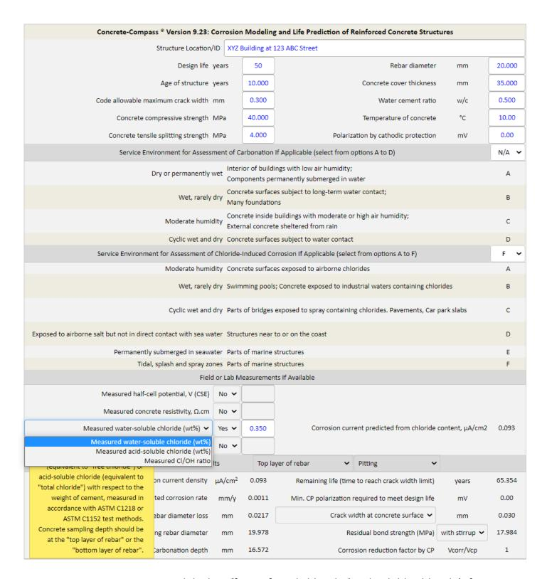
Figure 5 Concrete-Compass models the effects of total chloride (acid-soluble chloride), free chloride (water-soluble chloride), and CI/OH ratio on the corrosion rate.
