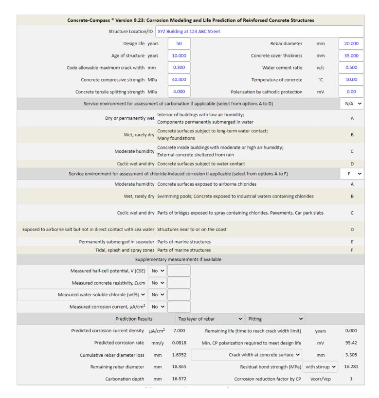
Figure 6 Concrete-Compass predicts concrete corrosion, crack width and remaining life of RC structures in accordance with BS EN 206 concrete exposure class.
