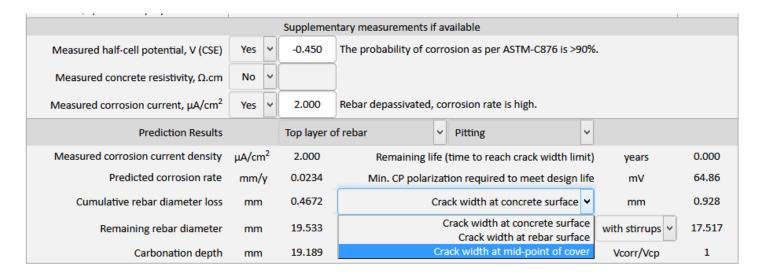
Figure 9 Concrete-Compass predicts the crack width at different depth of concrete cover.
