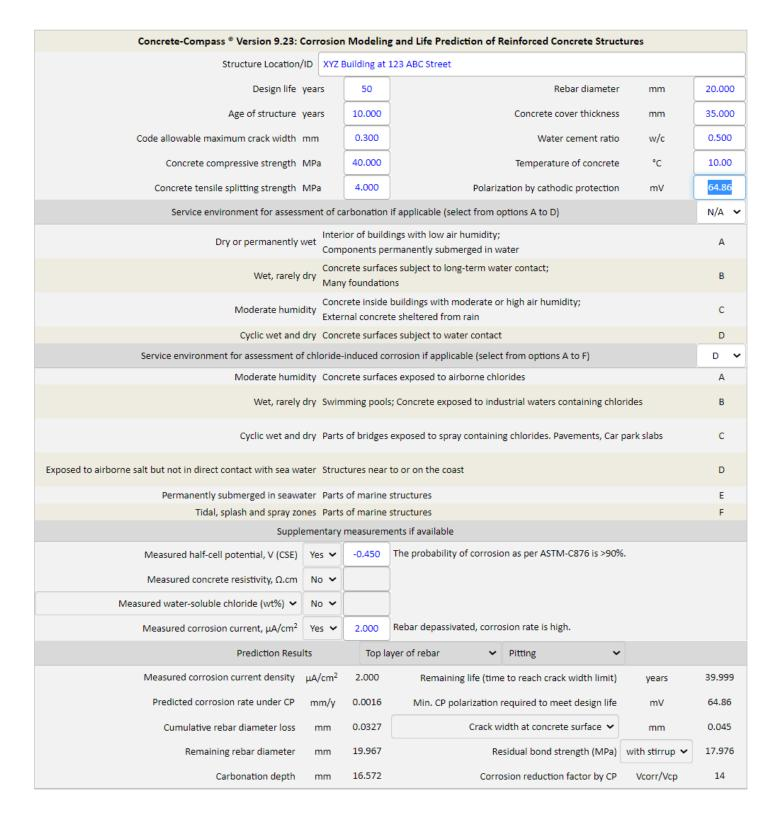
Figure 2 Concrete-Compass predicts concrete corrosion, crack width, bond strength, and cathodic protection requirement.
