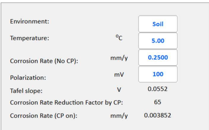
Figure 3 Assessing the degree of CP protection using CP-Compass software
