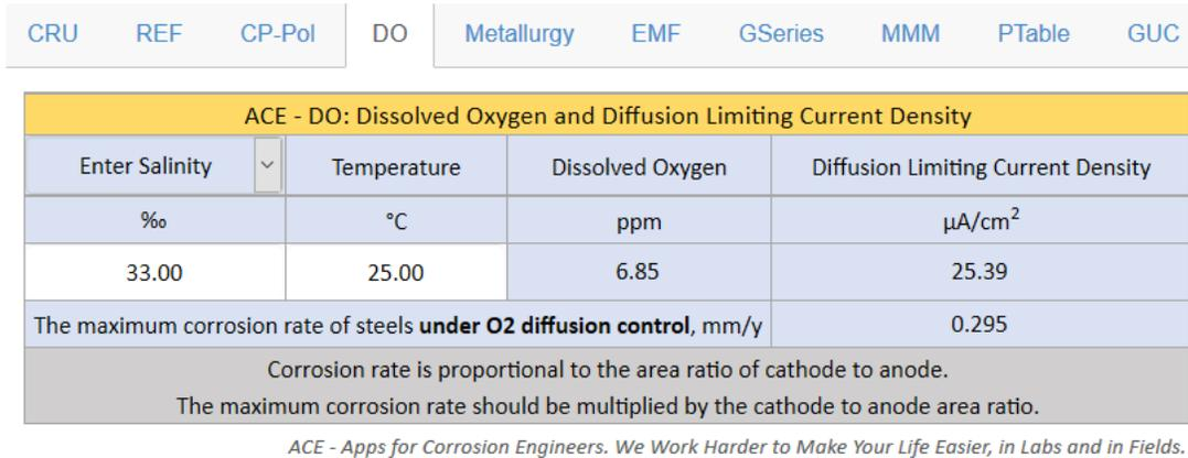
Figure 8 Calculation of Dissolved Oxygen in Waters at a Specified Temperature.
