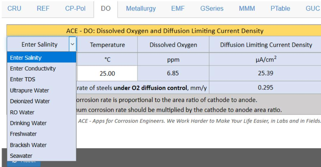
Figure 9 Calculation of Dissolved Oxygen and O2 Diffusion Limiting Current Density in Waters at a Specified Temperature.
