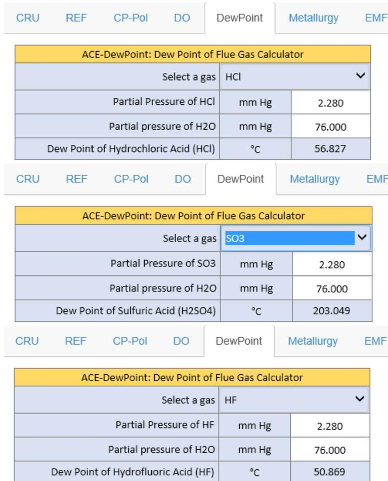
Figure 10 Predicting Dew Point of Flue Gas
