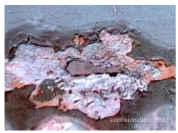
What alloys are susceptible to exfoliation? Aluminium alloys are susceptible to exfoliation corrosion. The photo above shows an aluminum alloy exposed to tropical marine environment. Also note the paint failures caused by corrosion of aluminum at the coating/aluminium interface.
