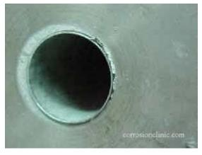
In this photo, a type 316 stainless steel tube and tube sheet from a heat exchanger in a seawater reverse osmosis (SWRO) desalination plant suffered crevice corrosion due to the presence of crevice (gap) between the tube and tube sheet.
