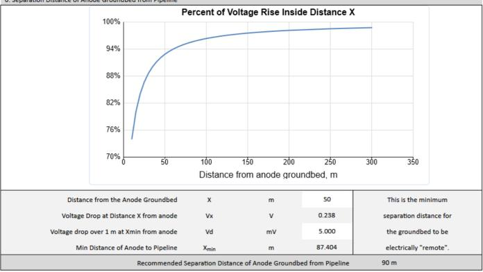
Current and potential attenuation are calculated automatically to give you the most realistic estimation of the number of anode groundbeds required (see plots under Section 3 above).
